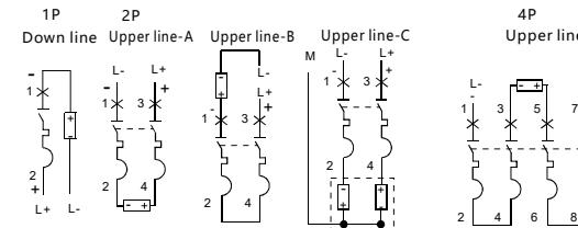
wiring instructions : 1 L+:positive pole, L-: negative pole; 2 +: breaker positive, -: Breaker negative;
